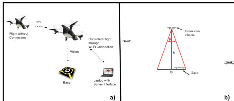
**Figura 1. a) Landing/take-off and recharging model using GPS and drone image processing. b) Calculation of the control transition height, below this height control is transferred from the drone to the recharging base.**
