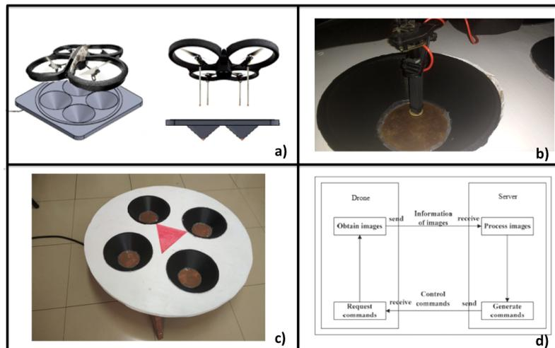
**Figura 2. a) Representation of the drone approach and contact if the drone feet with metallic contacts at the base. b) Adaptation of the contacts on the drone feet with the metal contacts on the base. c) Prototype of the recharge base developed for landing and recharging of an ArDrone. d) Representation of communication between drone and server.**
