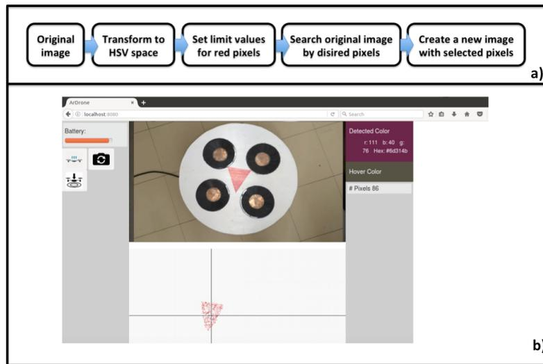
**Figure 3. a) Algorithm for color detection and image processing. b) Application main screen.**
