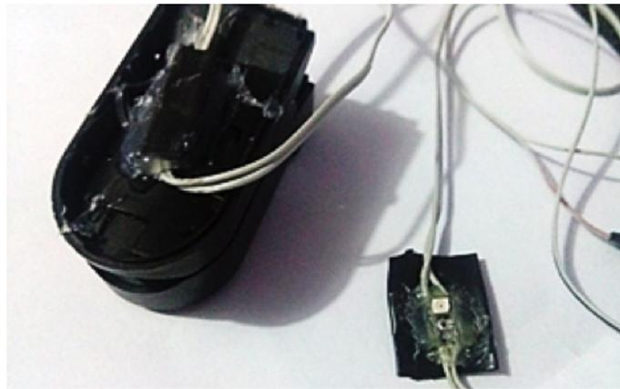
**Figura 2. Finger (a) and wrist (b) sensors prototypes.**
