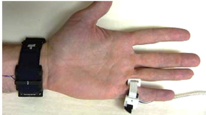
**Figura 1. Arrangement of the PPG sensors to measure PTT.**
