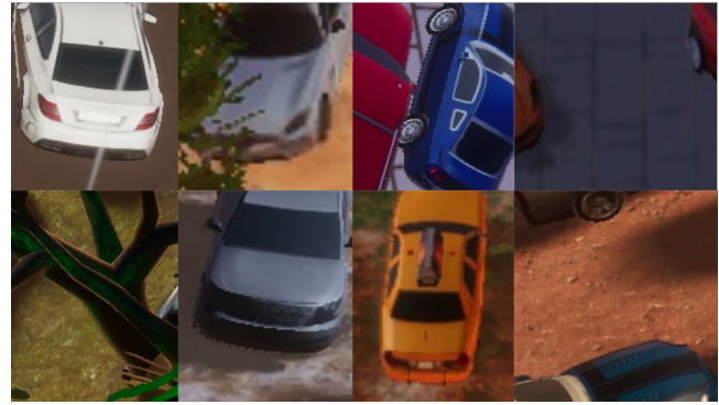
Figure 4: Example of parking spaces segmented into rotated rectangles. The spaces are labeled as either Occupied or Empty.
