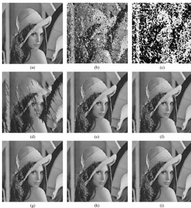
Figure 6: Filtering results for the Lena image corrupted by 80% salt-and-pepper noise: (a) free-noise image, (b) MF, (c) DWMF, (d) BPDF, (e) SMF, (f) AMF, (g) NAFSM, (h) MDBUTMF, (i) DAMF [27].
