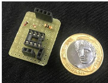
Figure 6 – DIY Timer with IC555 mounted on 2.5cmx3.0cm circuit board.
