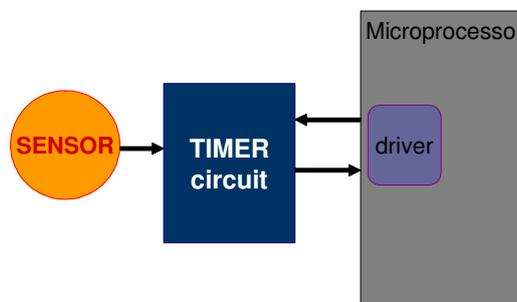
Figure 1 - Scheme of a digital sensor with a timer circuit.
