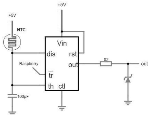
Figure 3 - Temperature sensor based on timer circuit based on IC555.
