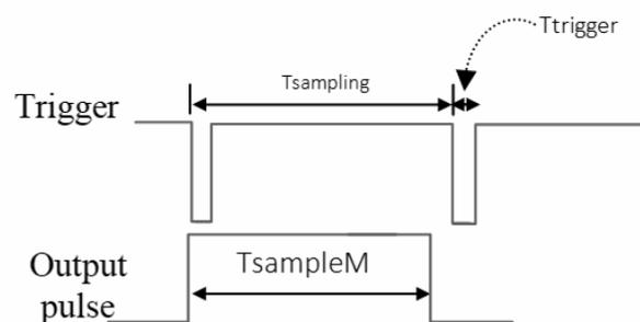
Figure 2 - Timing signal diagram.
